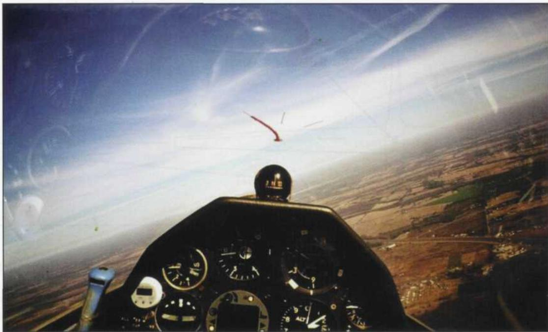
*Ventus A instrument panel and canopy view during a gentle right turn at 43 kts, when the yaw string angle is momentarily at almost 20 degrees on the high side of the turn. Author's Ventus thermaling experience showed that the yaw string angles normally varied between about 10 and 20 degrees on the high side when keeping the skid ball at the advocated 1/2 ball width on the low side of center. Unfortunately, I forgot to power the electric turn indicator.*
