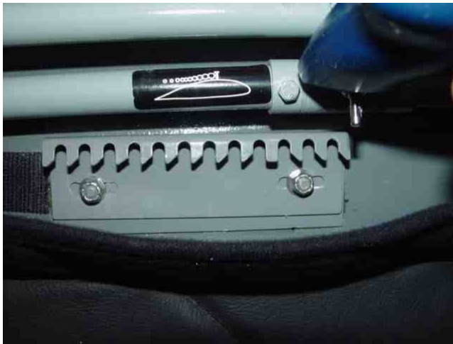
Figure 8 Piggott-hook example - pin on spoiler handle engages slots in plate (John Morgan)
