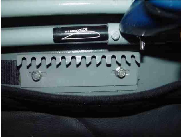
**Figure 8 Piggott-hook example - pin on spoiler handle engages slots in plate (John Morgan)**
